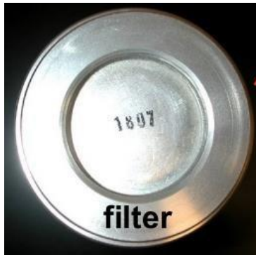
fig 3: aluminum filter attached to the tube head
