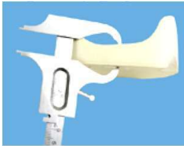
Figure (3-33): minimum thickness for the base of cast 11-15 mm.
