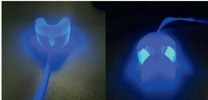
The intraoral device delivers light at an infrared frequency that penetrates the soft tissue over the alveolar bone
